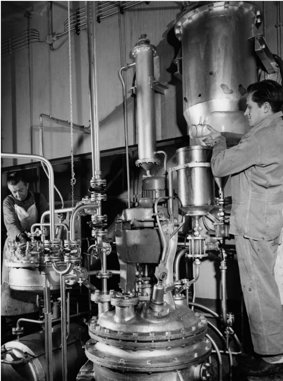
Technicians busy at the distillation of Postafene antihistamines products at the Berkendael laboratory. (ca. 1958) Courtesy of UCB Company Archives.
